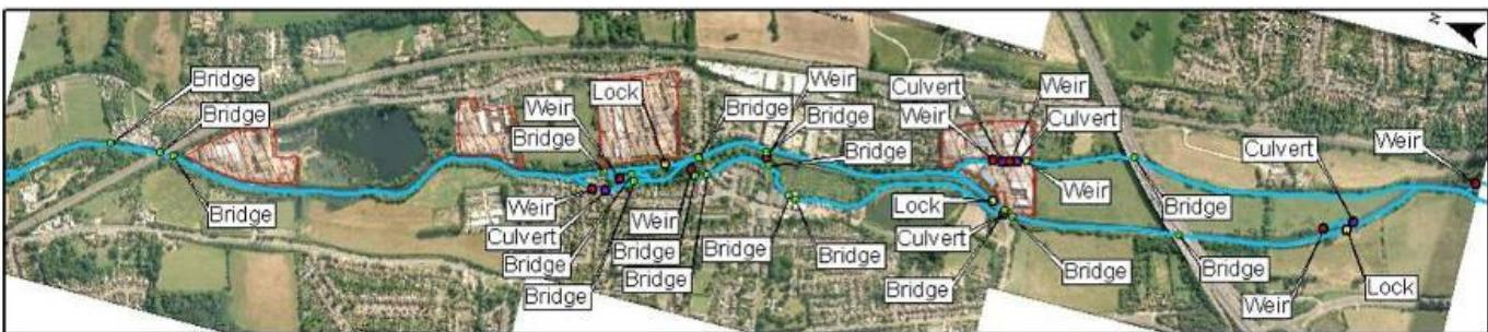
In selected locations the iSIS channel was augmented to include floodplain, modelled as either extended cross sections or Reservoir Units. The choice of floodplain unit was based on the hydraulic characteristics of the floodplains, e.g. flow direction, terrain characteristics and location of development areas.
