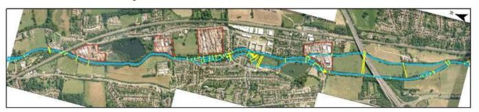
Structures such as bridges, weirs and locks were incorporated into the model using appropriate iSIS units. The iSIS unit parameters were obtained from the survey data. The structures are shown in Figure 2.4.
