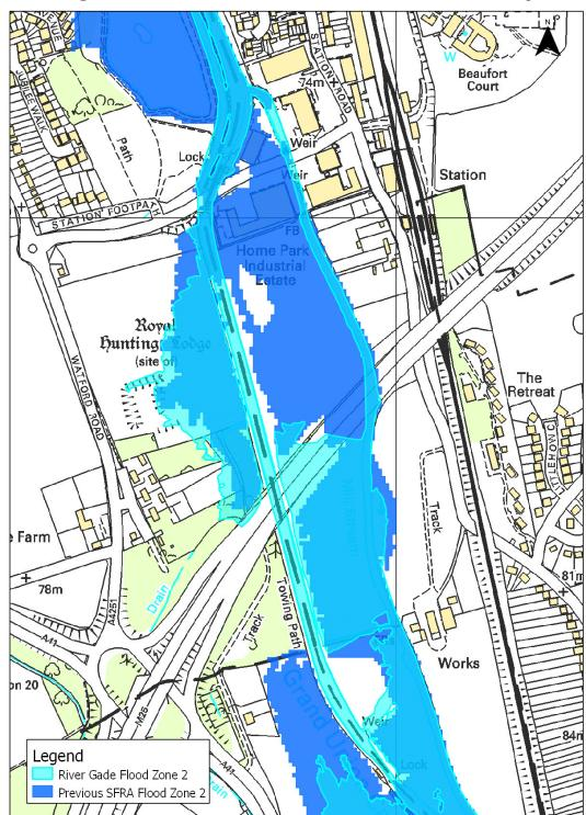
**Figure 4-4: Flood Zone 2 at Mill Lane**
