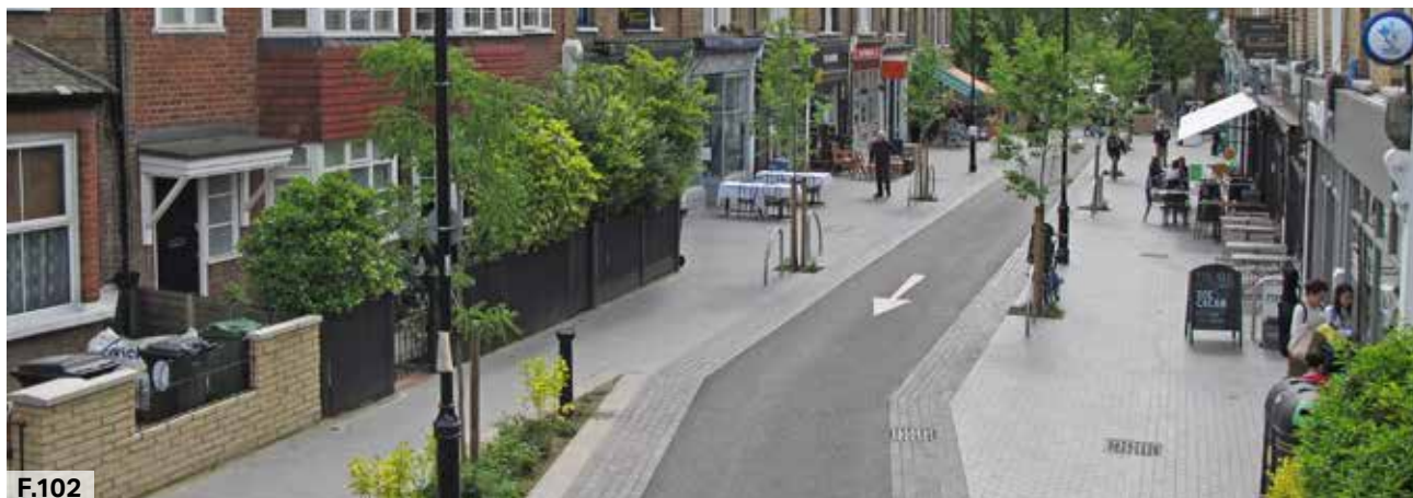
Figure 102: Shared surface with carriage and pavement on the same level. The shared surface can be used by all public realm users such as vehicle, pedestrian and cyclists. Trees can soften the area and improve the biodiversity, Walthamstow Village
