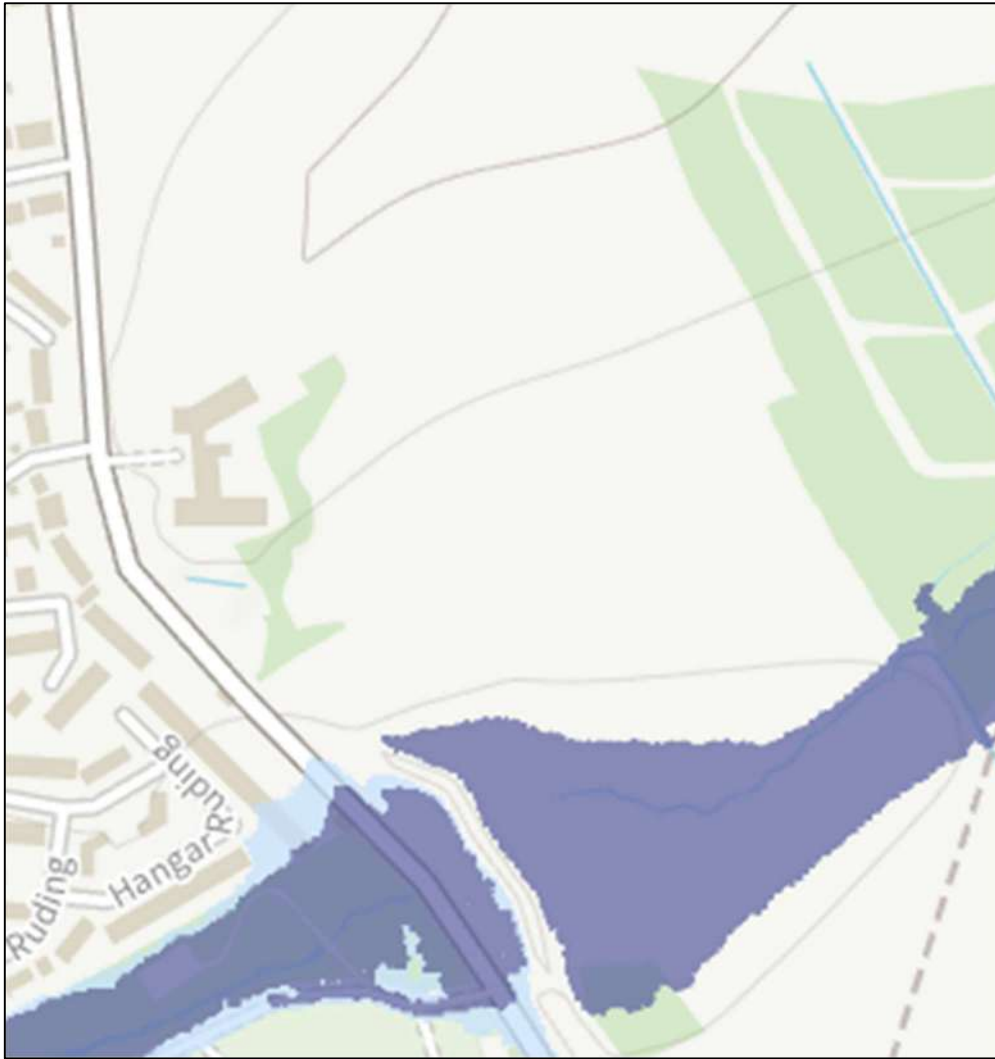
Figure 4-5: Groundwater Flooding Extents (Source: South West Hertfordshire Level 1 SFRA Appendix A by JBA Consulting)
