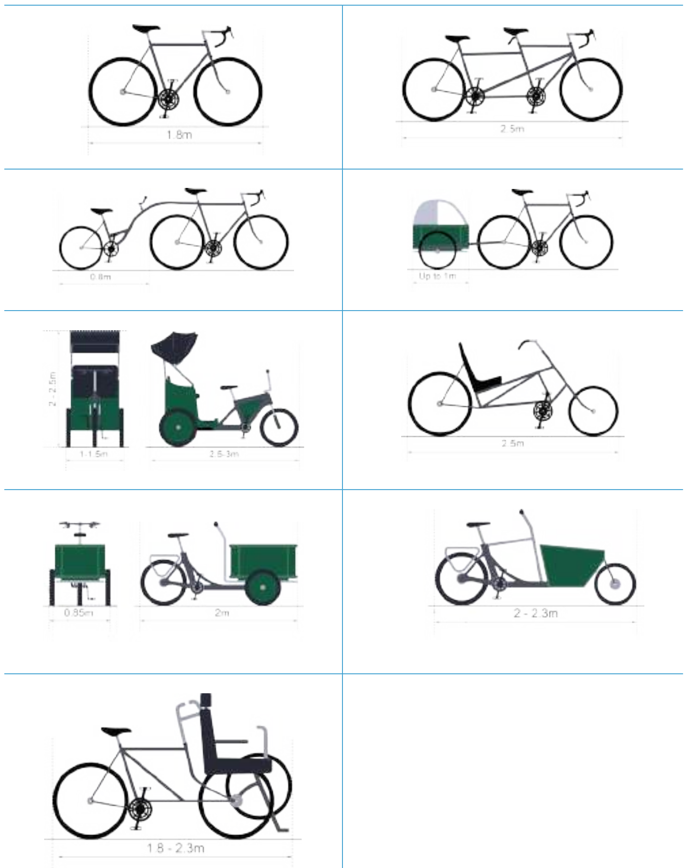
Figure 5.2: Typical dimensions of cycles
