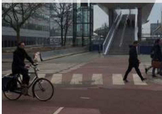
Figure 10.55: Cycle lift and wheeling ramps, Utrecht Station – most people use the ramps on the stairs because they are quicker but the lift meets the needs of people who cannot use them. (Note that the road markings do not comply with UK regulations.)
