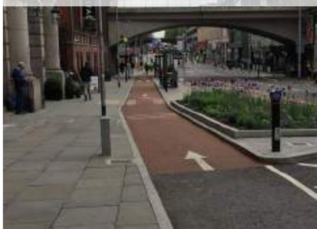
Figure 9.4: Cycle lane to cycle track transition
