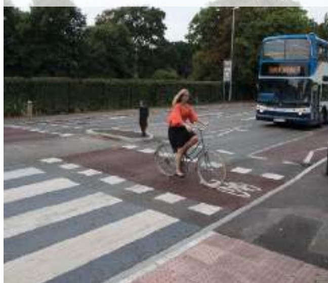
Figure 10.4: Parallel crossing with refuge
