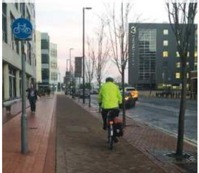
Figure 6.13: Double TSRGD diagram 1057 symbols on one way stepped cycle track, Cambridge
