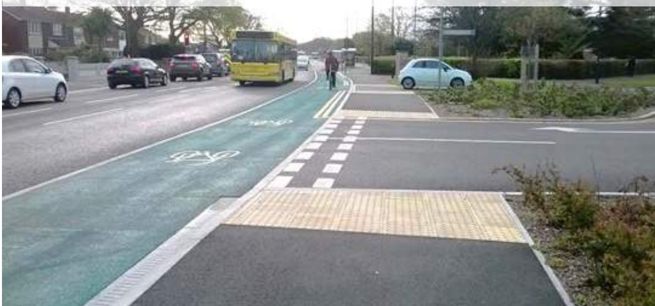
Figure 10.17: No setback crossing with design priority, – Bournemouth
