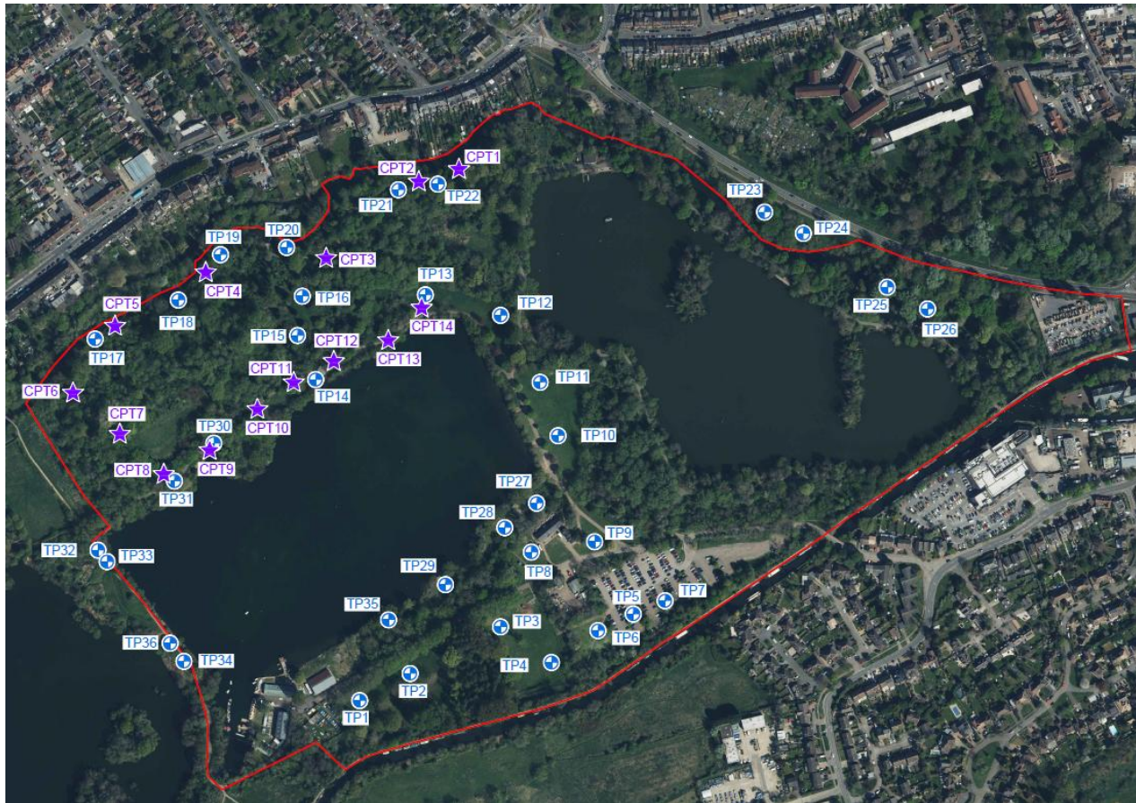
Site investigation locations for Trial Pits and Cone Penetration Testing
